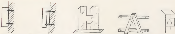
A. Mounted flush to wall. B. Projected on sleeves. C. Free standing on bar. D. Mounted to bars on back. E. Keyhole slots.
